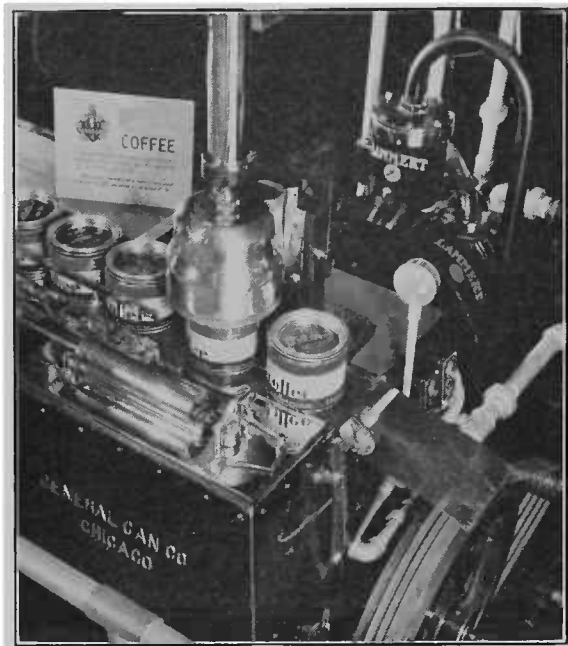
A GENERAL CAN COMPANY COFFEE VACUUM CLOSING MACHINE IN OPERATION
